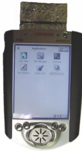
Figure 6.2.: iPAQ with its wireless card wrapped in aluminium foil
