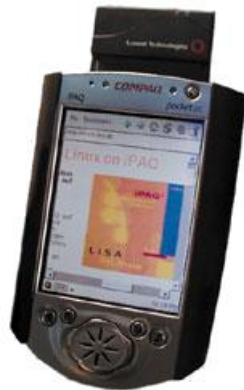
Figure 4.4.: Compaq iPAQ with 802.11b network card running Linux
